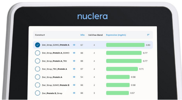
Figure 1. Expression and purification characterization. The instrument reports on expression and purified yield (mg/mL or \mu\text{M} ) to inform on the most favorable construct and cell-free blend.
